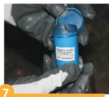
7 Open the lid of the thermowelding box
