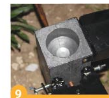
9 Insert the metal plate hole of the mould.
