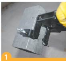
1 Connect the thermoweld mould with thermowelding plier
